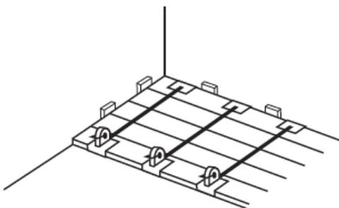
B. Typical: Every 3"-4" with staples, every 4"-6" with cleats, and within 1"-2" of end joints. Use appropriate size fastener for top nailing first row, last row and any area where blind nailer will not fit.
